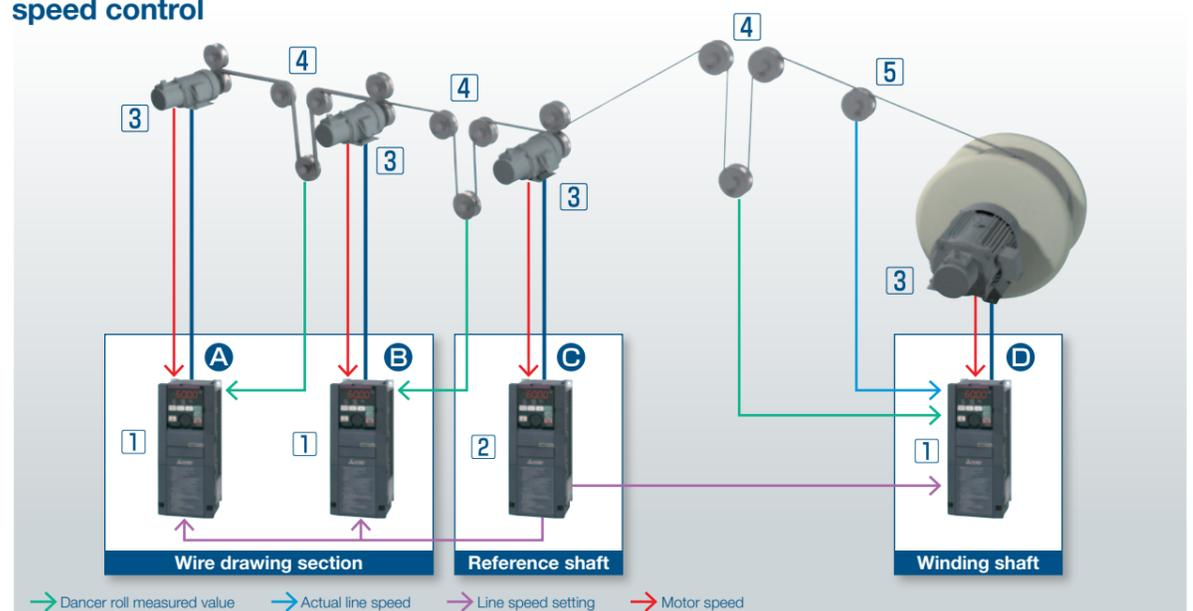
The wire drawing section pulls the wire at a constant speed to make the wire thinner. For the winding shaft, the inverter provides dancer feedback speed control to keep the dancer roll position, achieving constant tension winding. In addition, using the winding diameter calculation function, the circumferential speed of the winding bobbin is kept constant.
