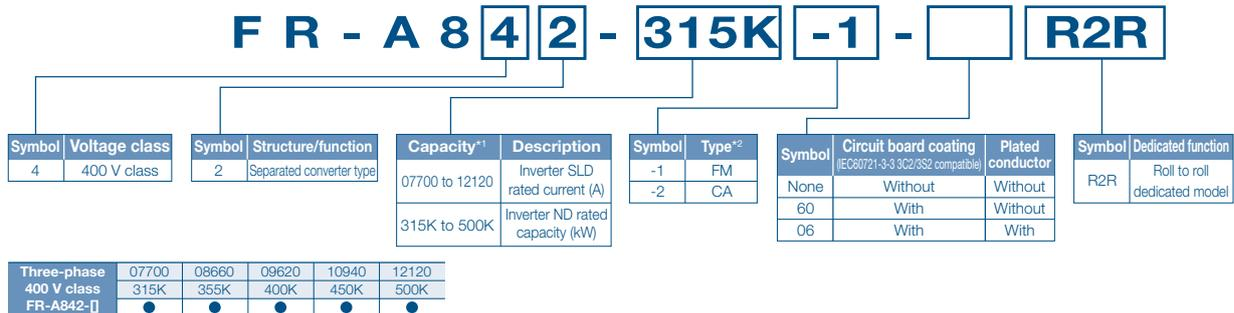
\*1 Models can be alternatively indicated with the inverter rated current (SLD rating).
