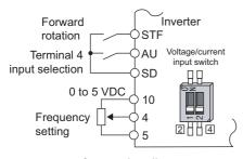
Connection diagram using terminal 4 (0 to 5 VDC)
