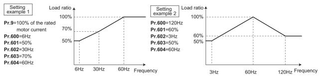
• When setting Pr.600, Pr.602, Pr.604 (Pr.692, Pr.694, Pr.696) to the same frequency, the following graph's upper level will be applied.
