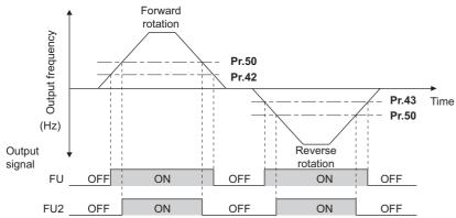
• For each signal, refer to the following table and assign the function by Pr.190 to Pr.196 (output terminal function selection)
