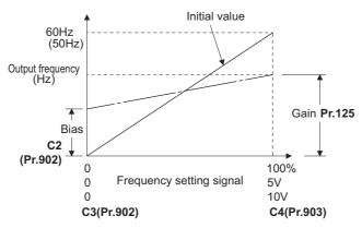
· Other adjustment methods for the frequency setting voltage gain are the following: adjustment by applying a voltage directly across terminals 2 and 5, and adjustment using a specified point without applying a voltage across terminals 2 and 5.
