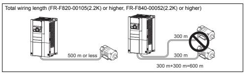
When driving a 400 V class motor by the inverter, surge voltages attributable to the wiring constants may occur at the motor terminals, deteriorating the insulation of the motor. In this case, take one of the following measures.
