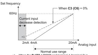
\*1 When the **Pr.573** ≠ "9999" and terminal 4 (terminal 2) is calibrated to 2 mA or less with **C2 (Pr.902) (C5 (Pr.904))**, analog input frequency that is 2 mA or less will become input current loss, thus it will not be as the bias setting frequency.
