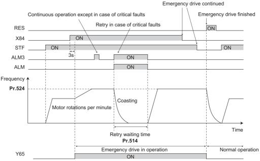
• When the electronic bypass during emergency drive is activated (CS signal is turned ON) (when the switchover to the commercial power supply during emergency drive is enabled)
