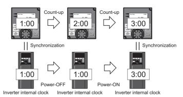
• When the FR-LU08 is connected to the inverter, the internal clock of the inverter can be synchronized with the clock of FR-LU08. (Real time clock function)
