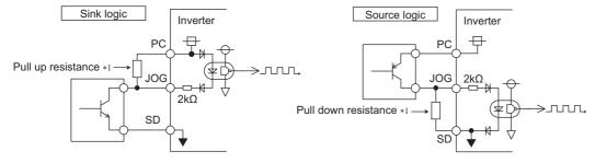
\*1 When the wiring length is long with open collector outputs, the influence of stray capacitance causes the pulse to flatten out and prevents the input pulse from being recognized.
