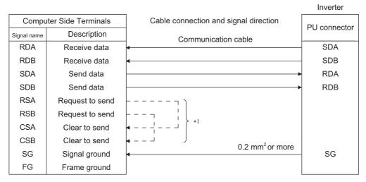
Make connection in accordance with the Instruction Manual of the computer to be used with. Fully check the terminal numbers of the computer since they vary with the model.
