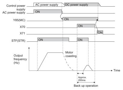
· Operation example at the time of power failure occurrence 2 (when the AC power supply is restored)
