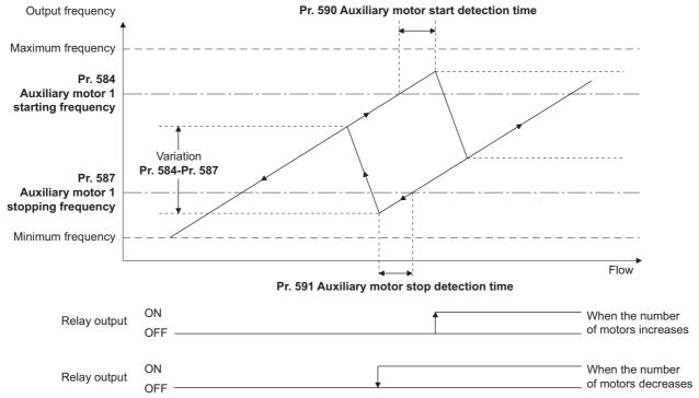
• Switchover timing at a start (stop) of an auxiliary motor 1 in the direct system (**Pr.579=**"2") and alternative direct system (**Pr.579=**"3")
