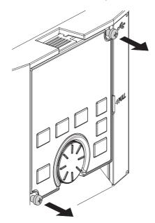
Press the upper edge of the operation panel while pulling out the operation panel.
