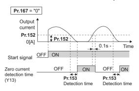
\* When the output is restored to the Pr.152 level, the Y13 signal is turned OFF after 0.1 s.
