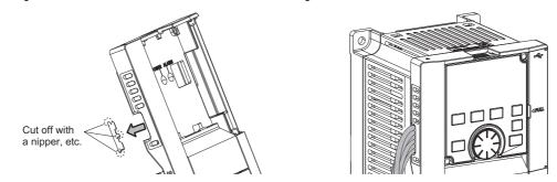
· When the FR-F820-01540(37K) of higher, or the FR-F840-00770(37K) or higher is used with a plug-in option, lead the wires on the left side of the plug-in option for wiring of the RS-485 terminals.
