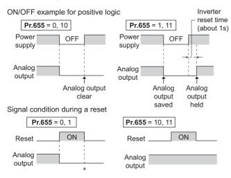
\* When Pr.655 = "1", the signal condition saved in EEPROM (condition of the last power OFF) is applied.
