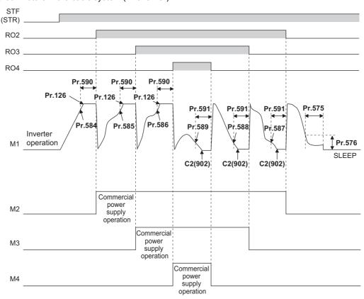
• When using two motors in the alternative system (Pr.579="1")
