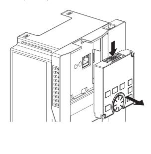
To reinstall the operation panel, align its connector on the back with the PU connector of the inverter, and insert the operation panel. After confirming that the operation panel is fit securely, tighten the screws. (Tightening torque: 0.40 to 0.45 N·m)
