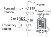
Connection diagram using terminal 2 (0 to 5 VDC)
