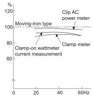
Example of measuring inverter output current
