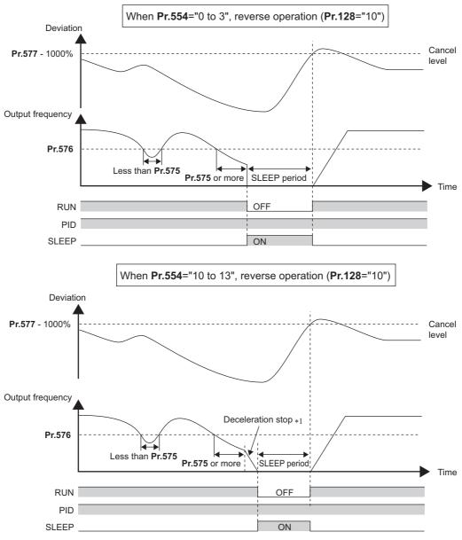
\*1 When the PID output shutoff release level is reached during a deceleration stop, output shutoff is released, operation is re-accelerated and PID control is continued. During deceleration **Pr.576 Output interruption detection level** is invalid.
