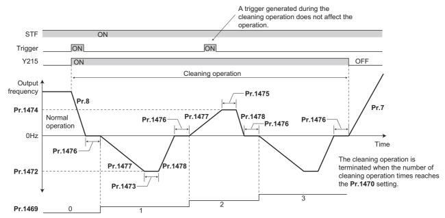
· When the number of times of cleaning operation is an odd number, the operation in the opposite direction to the start command is performed. When the number of cleaning times is an even number, the operation in the start command direction is performed.
