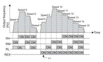
When RH, RM and RL is set to OFF and REX is set to ON when "9999" is set to Pr.232 Multi-speed setting (speed 8), the inverter runs by the frequency set to Pr.6.
