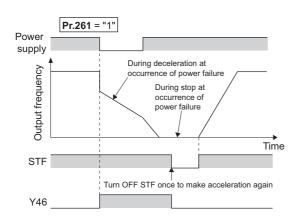
· Even if power is restored during deceleration triggered by a power failure, deceleration stop is continued after which the inverter stays stopped. To restart operation, turn the start signal OFF then ON again.
