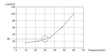
When the load reference is not set for five points, the load characteristics value is determined by linear interpolation of the set load reference values only. If there is only one load reference setting, the set load reference is used as the load reference all through the range.
