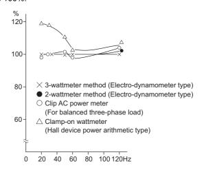
Example of measuring inverter output power
