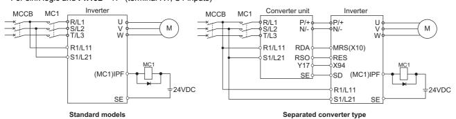
• For sink logic and Pr.192="17" (24 V external power supply input)
