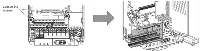
2) Be careful not to bend the pins of the inverter's control circuit connector, reinstall the control circuit terminal block and fix it with the mounting screws.
