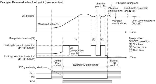
Details of the two-position ON/OFF operation
