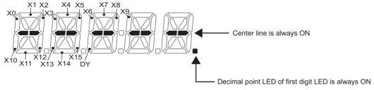
• The decimal point of the second digit on the LED will light for the output option terminal monitor (Pr.52 = "57").
