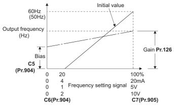
· Other adjustment methods for the frequency setting current gain are the following: adjustment by applying a current through terminals 4 and 5, and adjustment using a specified point without applying a current through terminals 4 and 5.
