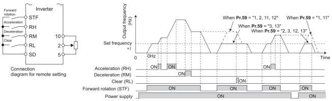
\*1 External operation frequency (other than multi-speed) or PU running frequency
