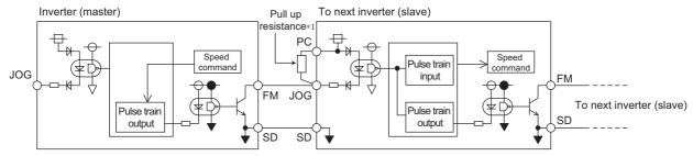
\*1 When the wiring length between FM and JOG is long, the influence of stray capacitance causes the pulse to flatten out and prevents the input pulse from being recognized. When the wiring length is long (10 m or longer of shielded twisted pair cable with a recommended cable size of 0.75 mm²), connect the terminal JOG to the terminal PC by an external pull-up resistance. The table below shows the reference resistance values for wiring length.
