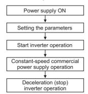
· Signal operation after setting parameters
