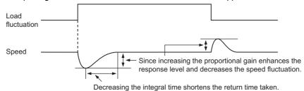
JM: Motor inertia Actual speed gain = Speed gain of a single motor  $\times$ JM + JL JL: Load inertia converted as the motor axis inertia
