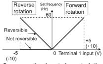
**Compensation input characteristics** when STF is ON
