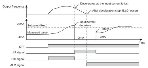
• The analog input current is restored during deceleration under PID control (reverse action)
