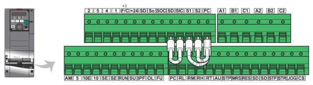
\*1 This terminal operates as the terminal FM for the FM type, and as the terminal CA for the CA type.
