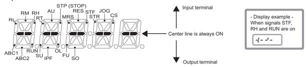
• The decimal point of the first digit on the LED will light for the input option terminal monitor (Pr.52 = "56").
