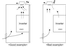
Arrangement of the ventilation fan and inverter
