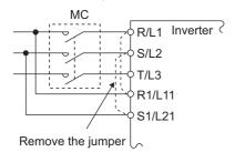
When a fault occurs, opening of the electromagnetic contactor (MC) on the inverter power supply side results in power loss in the control circuit, disabling the fault output signal retention. Terminals R1/L11 and S1/L21 are provided to hold a fault signal. In this case, connect the power supply terminals R1/L11 and S1/L21 of the control circuit to the input side of the MC.
