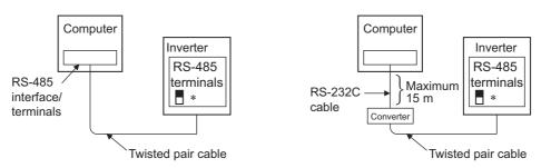
\*Set the terminating resistor switch to the "100  $\Omega$ " position.
