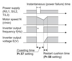
\* The output shut off timing differs according to the load condition.
